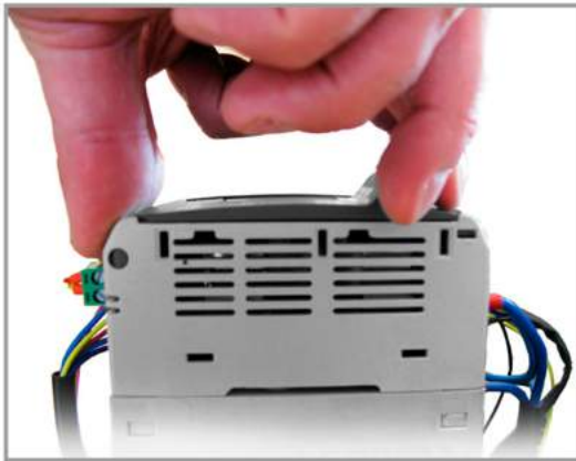
1. Open fuse holder by pulling the frontal cover
