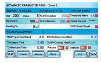
For each loop is available an advanced page with the following parameters and alarm. The parameters with light blue colour can be setted on this page. This page can be displayed touching the zone name on the main operating page. Touching the arrov keys, is possible to move to the next zone or to move on the previous zone.
